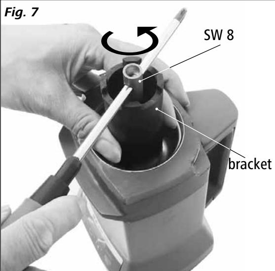
**Note:** When removing the **A10.2** Star-shaped beater, use the hooks on the bracket to hold the cutter. Then, the cutter can be taken out of the chamber (see **Fig. 9**, **Fig. 10**).
