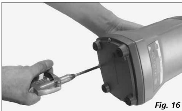
If there is heavy accumulation of dirt on this area, please wiped clean with a moist cloth. Never clean it in water or in a dishwasher.
