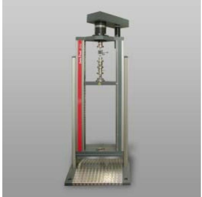
Figure: Table-top testing machine with torsion drive
