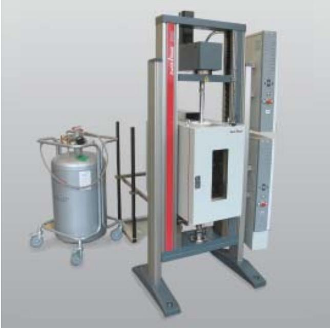
Figure: Table-top testing machine with torsion drive
