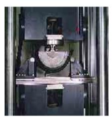
Bending testing device with sliding system
