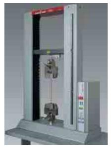
Materials testing machine BasicLine Z020
