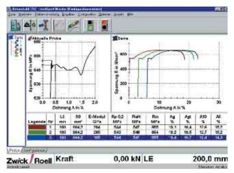
$\textit{testXpert}^{{\scriptscriptstyle 0}}\text{-}Screenshot:$  Tensile test on steel wire for the reinforcement of concrete with r- and n-value determination
