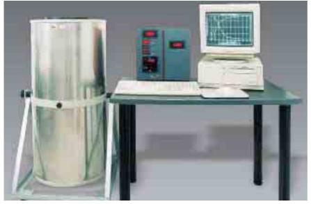
Heat-flow differential calorimeter ToniCAL concrete
