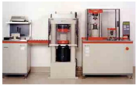
ToniPRAX with ToniNORM 3000 and specimen measuring device for cube tests
