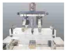
Transducer for measuring the bending deformation
