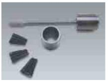
Specimens of reinforcement bars with clamping jaws
