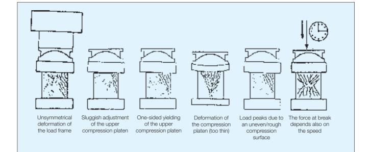
Different causes for a nonuniform load application on the specimen
