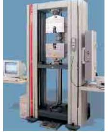
Materials testing machine Z100 with *testControl* PC variant
