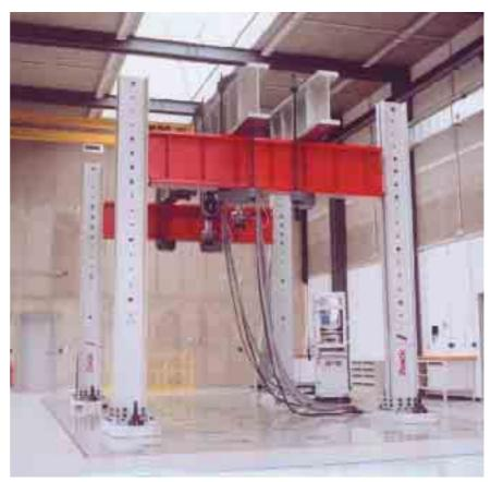
Component test system 1000 kN for the testing of supporting frameworks, large tubes etc. with a four-column load frame on an extremely rigid foundation plate made of reinforced concrete.
