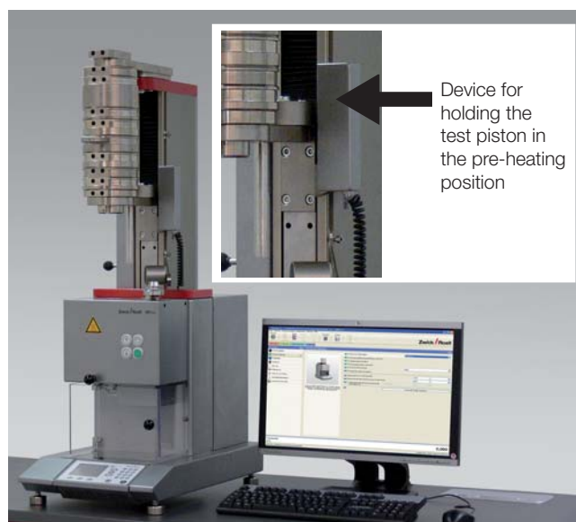
Fig. 3: Mflow with weight selector and device for holding the test piston in the pre-heating position
