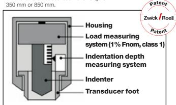
The patented hardness measuring head contains a load cell, a digital depth-measurement system (resolution 0.02  $\mu$ m), an indentor and a sensor foot in complete accordance with the Abbe measurement principle.
