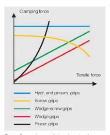
Fig 1: Dependence of the clamping force on the test load for different types of specimen grips
