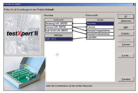
Fig 1: Full integration of a HB MGCplus in testXpert® II Small picture: Digital I/O box, additional with two output channels
