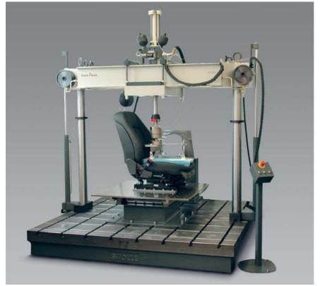
Fig 2: Servo-hydraulic test bench with hydraulically clamped and moveable crossboard. The actuator can be moved horizontally. (Fmax 100 kN)
