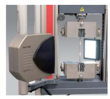
Fig 3: laserXtens with round specimen
