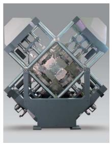
Fig 4: Fraunhofer Institut IWU Chemnitz, Germany: Biaxial tensile tests of metals
