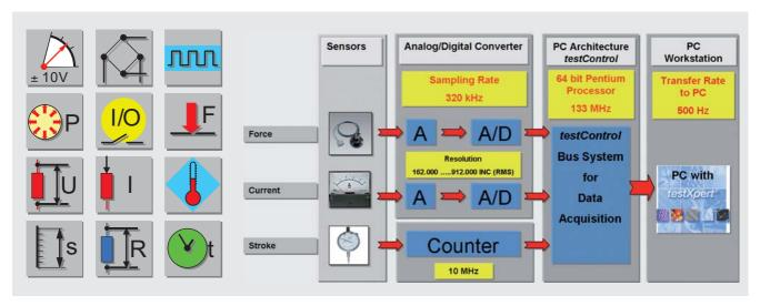
Fig 2: Analog and digital signals could be connected to  $\textit{testXpert}^{\texttt{@}}$  and testcontrol
