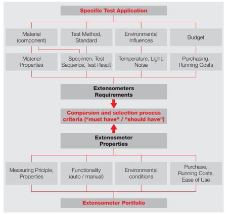
Fig 4: Selection process of extensometers
