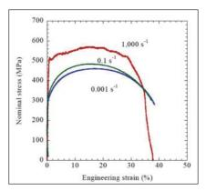
Fig 3: Materials characteristics depending on the loading rate
