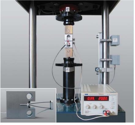
Fig 4: CT specimen in vibrophore (HFP)
