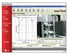
Fig 1: The video picture and the data curves are exactly synchronized
