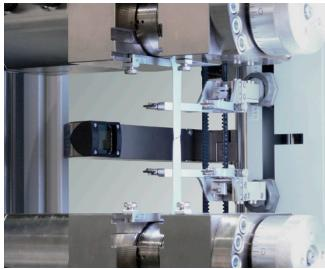
videoXtens' non-contact, high resolution transverse strain measurement allows determination of r-values to ISO 10113.
